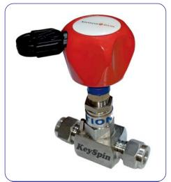
When the key is inserted in to the recess of the knob, the coded magnet engages the drive mechanism. Turning the locking head now turns the valve.
